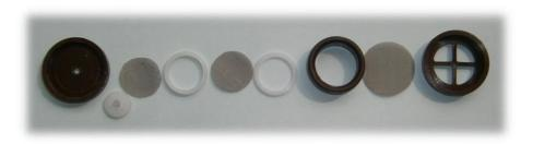
1. Wash all parts of passive samplers by tap waters. Rinse twice by deionized water. Leave on the air to dry. Do not dry by heat.
